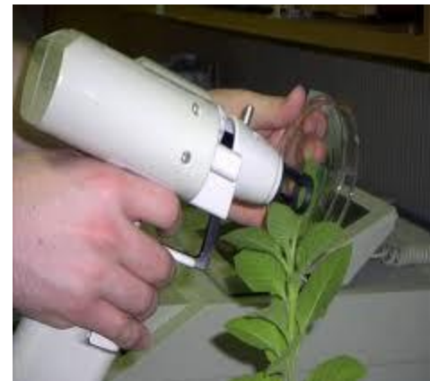
Gene gun Helios™ by BioRad is used to transfect cells in cultures and plant leaves
