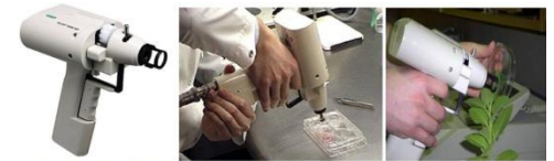
Gene gun Helios™ by BioRad is used to transfect cells in cultures and plant leaves
